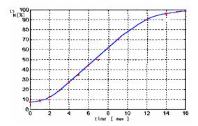
Figure 3: The variation of the isotopic concentration as a function of time obtained from experiments in the second separation column
