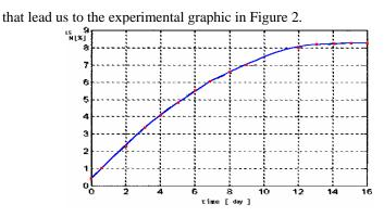
Figure 2. The variation of the isotopic concentration as a function of time obtained from experiments in the first separation column
