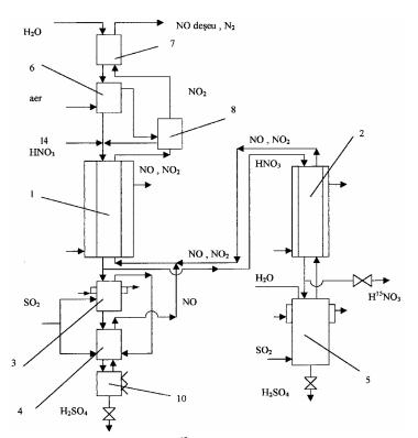
Figure 1. The installation for isotopic separation  $^{15}N$  through isotopic exchange NO, NO<sub>2</sub> – HNO<sub>3</sub>
