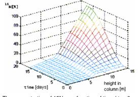
Figure 5. The concentration of 15N as a function of time (t = 0, ..., 16 days) and the height in the two columns (z = 0, 1, ..., 7m; z = 7, ..., 14m)
