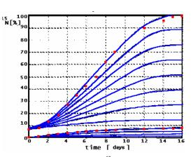
Figure 4. The concentration of <sup>15</sup>N as a function of time for different height in the two columns (0, 1, ..., 7m)
